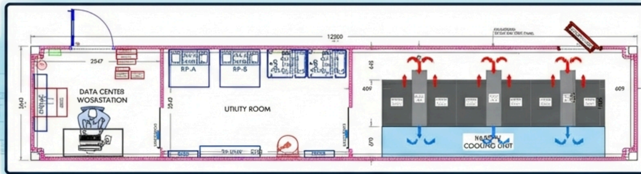
Single 40' Modular Data Center Pod (10kW x 6 Nos)
